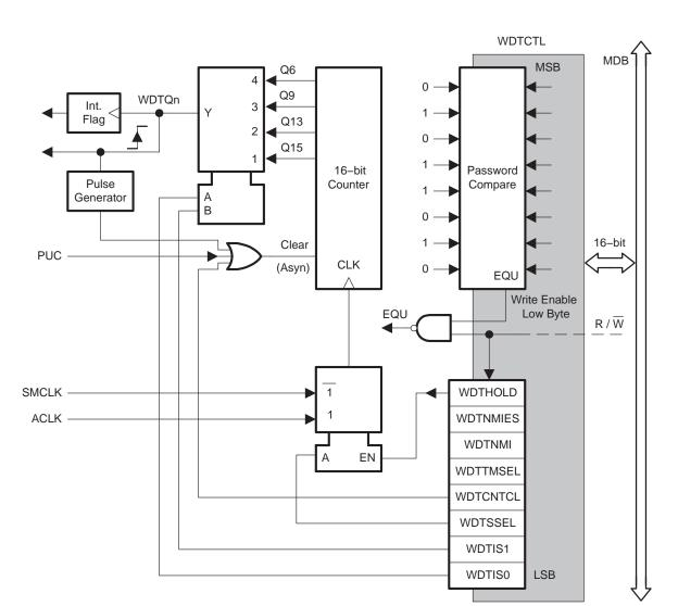
Figure 10–1. Watchdog Timer Block Diagram
